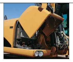
**Front Compartment.** The front compartment hood can be opened vertically, providing outstanding ground level access to the batteries, air-to-air after cooler, air conditioner condenser and the air cleaner filter.
