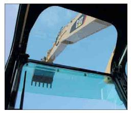
Viewing Area. To maximize visibility, all glass is affixed directly to the cab, eliminating the use of window frames. Choice of fixed or easy-to-open split front windshield meet operator preference and application conditions.
