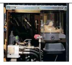
**New Auto-Lube System.** The new automatic lubrication system provides the optimal amount of grease to all the main lubrication points, including the bucket linkage. The lubrication interval can be adjusted through the monitor, and status messages for the auto-lube system are displayed.
