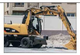
Variable Adjustable (VA) Boom. The VA boom offers improved right side visibility and machine roading balance. When working in tight quarters or lifting heavy loads, the VA boom offers the best flexibility.
