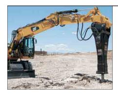
**Design.** Booms and sticks are welded, box section structures with thick, multiplate fabrications in high stress areas, for rugged performance and long service life.
