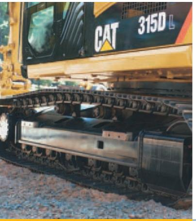
Caterpillar uses advanced engineering and software to analyze all structures, creating a durable, reliable machine for the toughest applications. More than 70 percent of the structural welds are robotic and achieve additional penetration over manual welds. These structural components and undercarriage are the backbone of the machine's durability.
